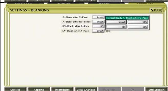
Note: Smart blanking is the equivalent to a 37.5 ms value, any device programmed to a positive LV Offset of 35 ms or less is not affected and not subject to the risks described in this letter.
