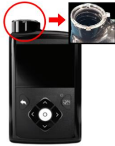
Image: Location of the retainer ring on the MiniMed™ 600 series insulin pump
