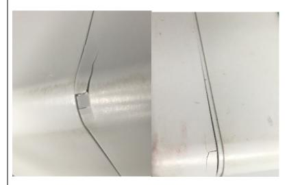
If the FRED Easy device shows cracks, impacts or deformation that could suggest that it has sustained a significant mechanical impact or contains a moving part, it should undergo maintenance.
