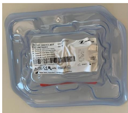
Picture 1: View of the deformed blister
