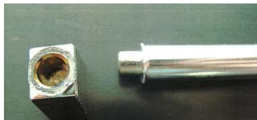
Picture 2: View of the issue with the straight shaft
